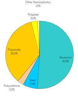
ID Mesh with aluminium base, aluminium ring armrests (43100100). Cover fabrics will be separated into synthetic materials and natural fibres, depending on the material.
