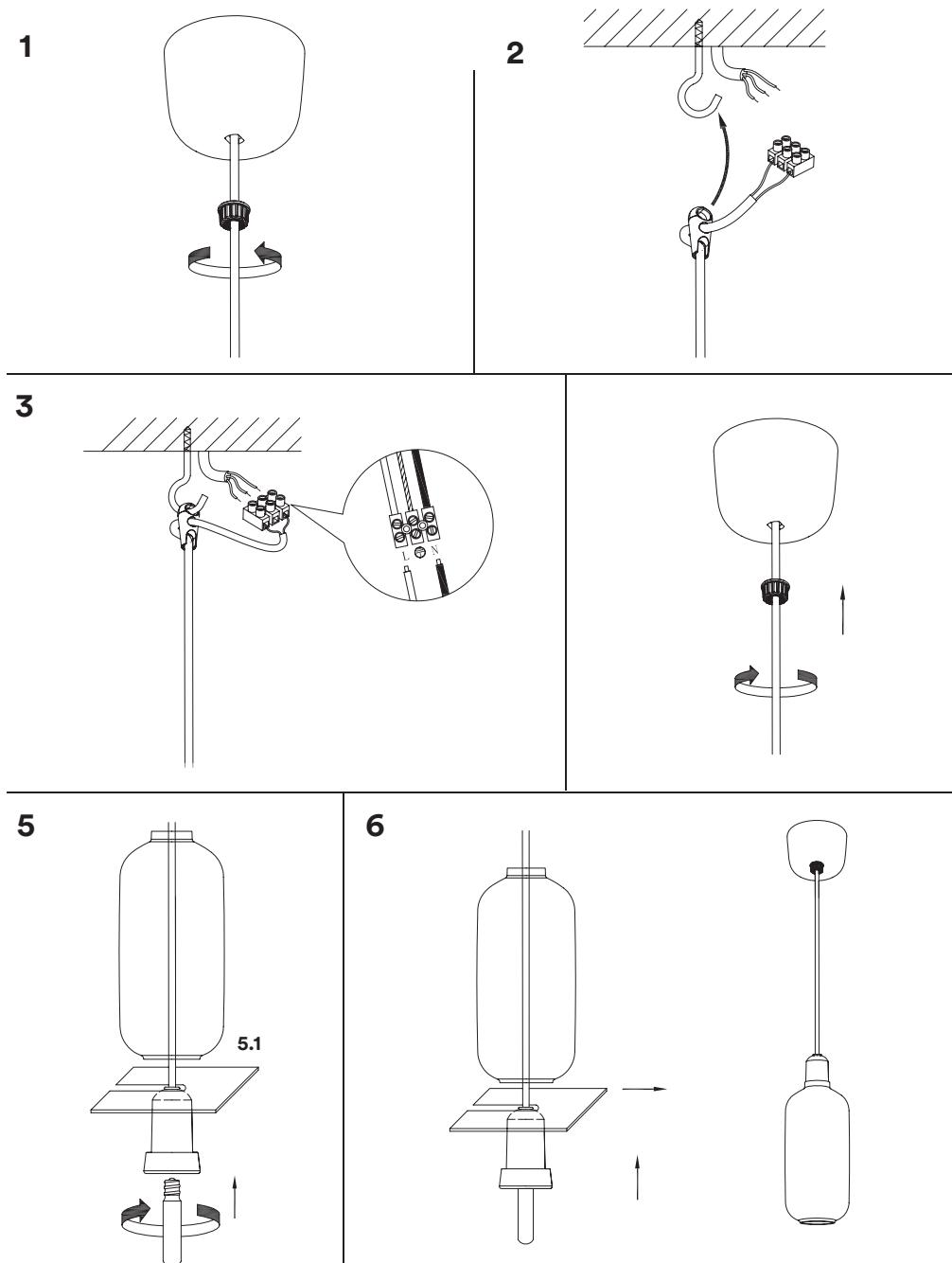
**5.1** Place the included cardboard piece between the socket and the lampshade to prevent it from any damage while inserting the bulb.
